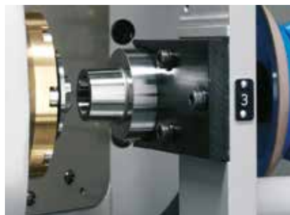
The eight-station wheel changer integrated into the S22 as a standard feature.
