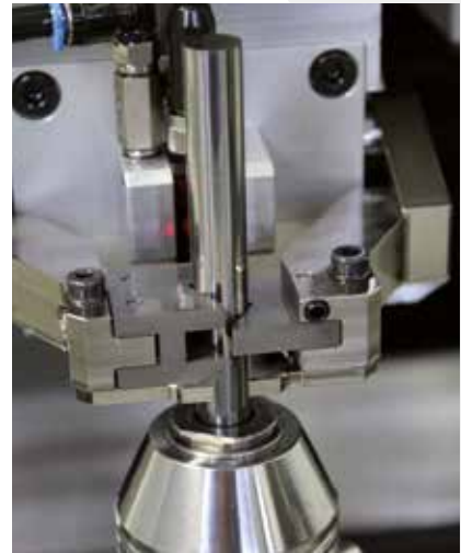
Reliable changing into hydraulic expansion chuck.
